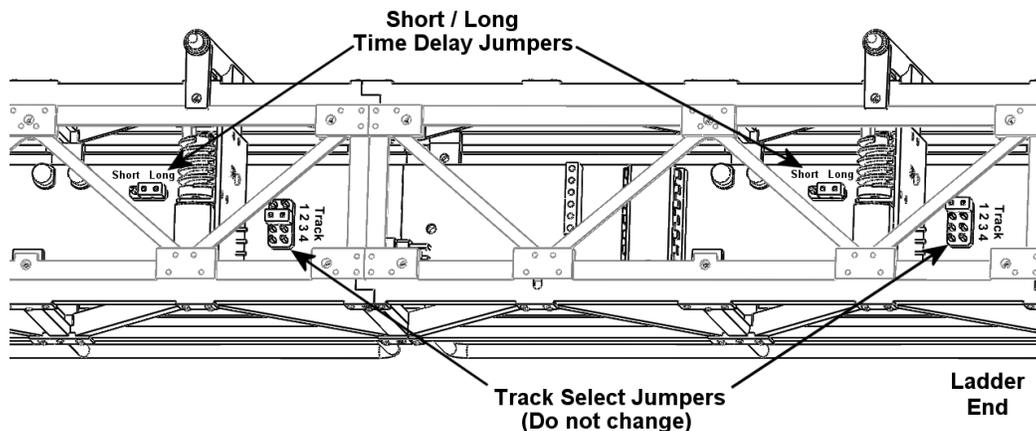
**OPTION** – If the output wire of a signal (or isolated rail) down-track is connected to one of the input wires of the signal bridge, the signal for that track input will hold on stop until the down-track signal is clear, then the signal bridge signal will cycle back to clear.
